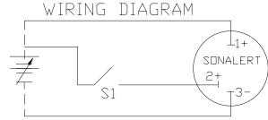
IF S1 IS OPEN, UNIT IS CONTINUOUS IF S1 IS CLOSED, UNIT IS PULSATING
